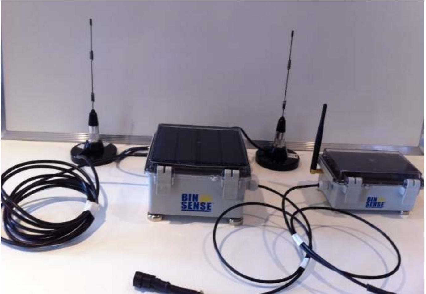
“BIN SENSE” Wireless Grain Monitoring System – Master & Remote Unit w/hinged Solar Lids
