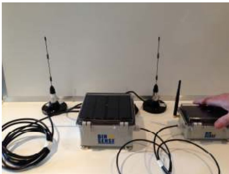
"BIN SENSE" Wireless Master & Remote Unit
